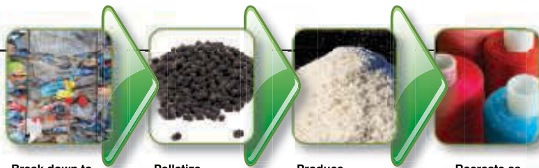
FIGURE 3. The proprietary chemical process behind Teijin's Eco Circle technology creates recycled polyester fibers that are of equal quality to polyester produced from all-new materials
