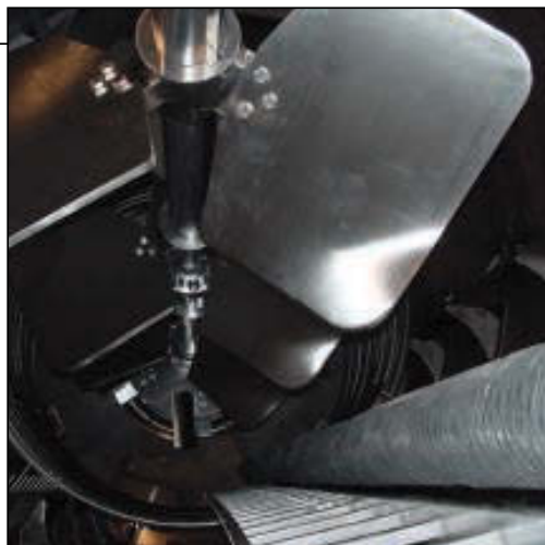
FIGURE 2. This configuration of a combined radial- and axial-impeller system is typical to provide mixing in an aerobic fermenter
